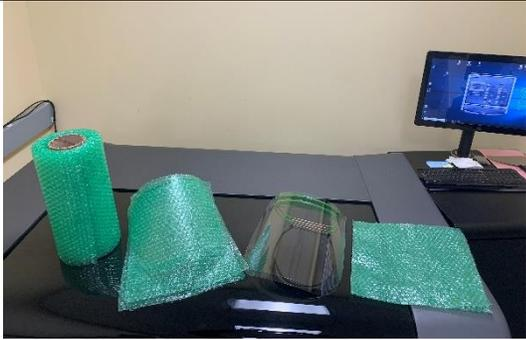
it over-top the shield so that you can stack the face shields in stacks of 10 to optimize packaging. The bubble wrap also protects the shields from obtaining any damage while being transported. Once a stack of 10 is made, there will be two stacks placed within a box which will then be given the green light indicating
