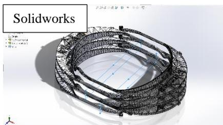
a print file was provided by Stratasys, however, as for the project, I had to try to replicate a close representation of what was used during the main production stage for that the original file was lost. To achieve this, I had to use a solid modeling computer-aided design program called Solidworks to create a part file then use the newly created part file to make an assembly. After looking at many photos of prints during the main production stage, the next step
